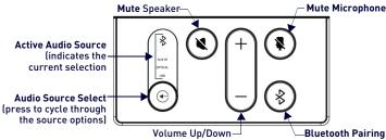
FIG. 8 ACV-2100 LEFT SIDE PANEL KEYPAD
