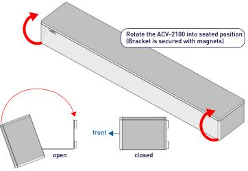
FIG. 6 ROTATING THE ACV-2100 INTO ITS SEATED POSITION
