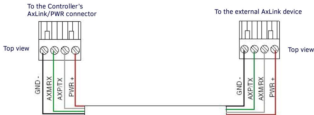
FIG. 56 Mini-Phoenix Connector Wiring Diagram (Direct Data And Power)
