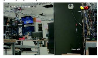
The length of the category cable affects the quality of the image. The above image has a 298-ft Cat 5 cable connected to the HD-TVI balun, with power passing through the balun.
