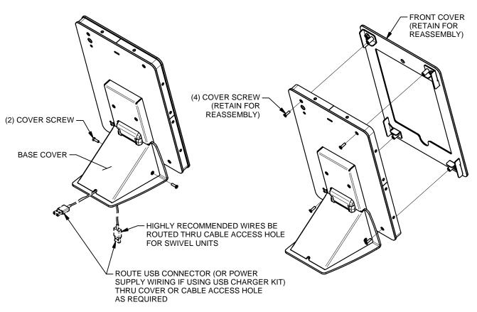
6. REASSEMBLE FRONT PANEL WITH IPAD. EXPLODED VIEW FOR REFERENCE. SEE BACK PAGE FOR FINAL ASSEMBLY.
