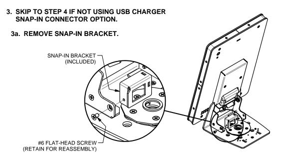
3b. INSTALL USB CHARGER SNAP-IN CONNECTOR ONTO SNAP-IN BRACKET. CONNECT USB END TO USB CHARGER.
