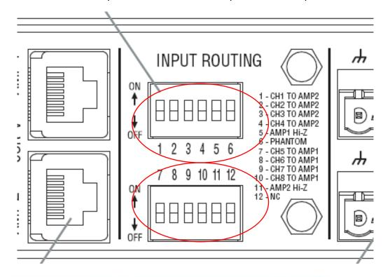
Step 2: 1-Channel CSMA. Locate the Hi-Z Configuration switch on the back of the mixer/amplifier. Turning this on will set the output of Channel 1 to Hi-Z or high impedance for 70volt or 100volt operation.
