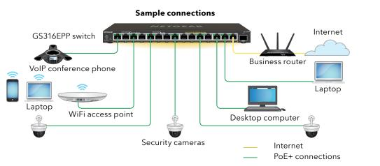
**NOTE:** We recommend that you use a Category 5e (Cat 5e) cable or higher-rated cable for Gigabit Ethernet connections.
