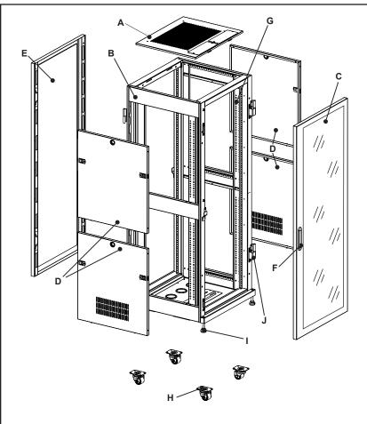
Rails accept 10-32 rack screws (40 included). Additional screws are available in a no-roll jar that includes 200 screws and nylon washers. (SR-SCREWS-200JAR)
