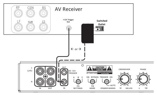
If the receiver does not have a 12V trigger output, using a 12V power supply plugged into a switched outlet on the receiver provides the same functionality.
