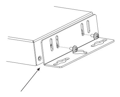
Attach the brackets provided to side panels of the device
