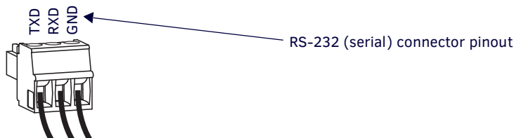
FIG. 34 Wire RS-232 ports for serial data transfer
