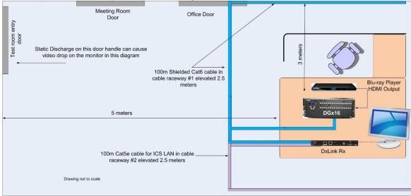
Figure 2 - Proximity ESD Event Test Diagram
