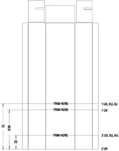
FIG. 32 High Voltage Isolator - Trim Template
