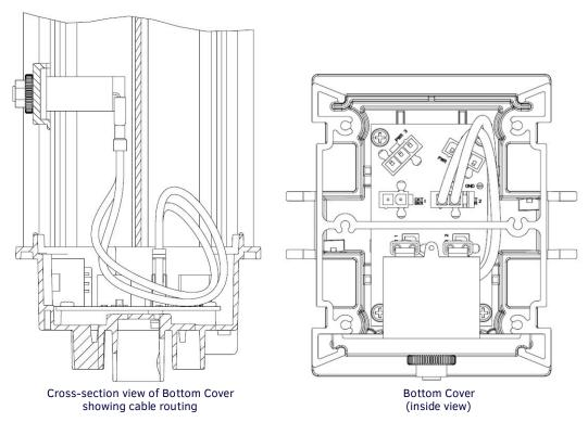
FIG. 11 Bottom Cover - Connect Each AC Power Module to the Power Inlet Assembly
