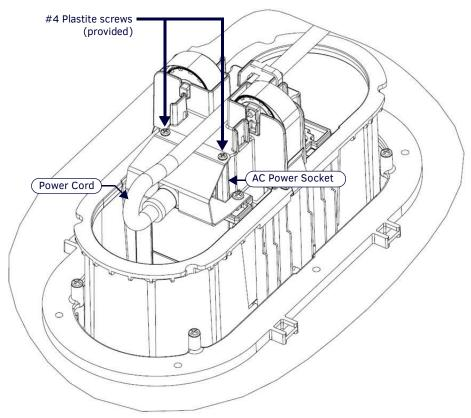
FIG. 21 Installing the Power Cord
