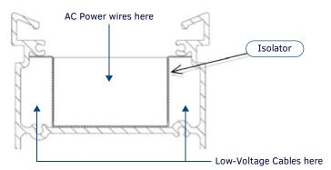
FIG. 31 High Voltage Isolator Cross Section
