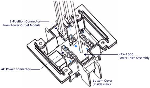
FIG. 26 HPX-1600 Bottom Cover - Connect Power Outlet Module to Power Inlet Assembly
