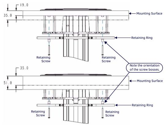
FIG. 8 Direction of the Screw-Bosses, Based On Surface Thickness (19mm vs. >19mm thick)
