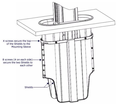
FIG. 22 Installing the Shields
