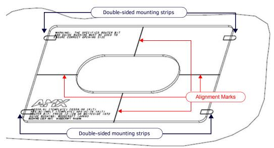
FIG. 5 HPX-AC-T Router Template
