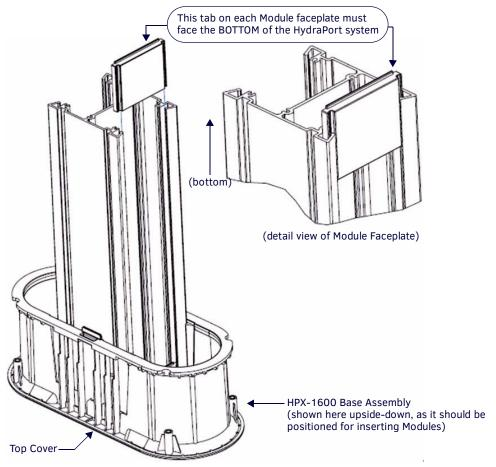
FIG. 10 Inserting Modules Into the HPX-1600 Base Assembly
