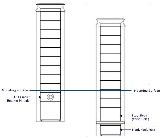
FIG. 12 Install Blank Modules at the Bottom of the System
