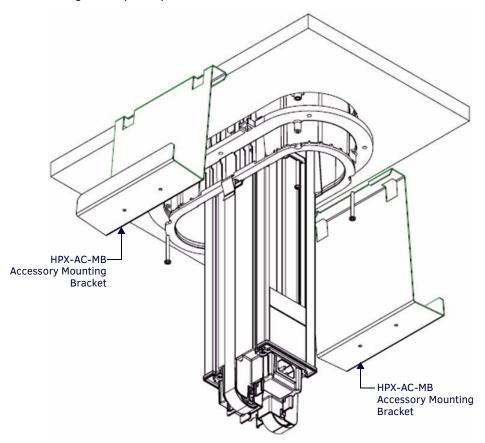
FIG. 19 Installing HPX-AC-MB Accessory Mounting Brackets
