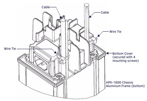
FIG. 15 Bottom Cover - Installed with Cables Exiting and Secured
