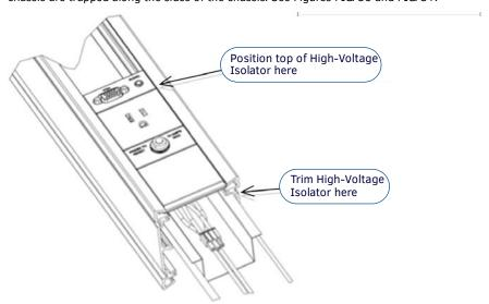
FIG. 30 High Voltage Isolator Installed
