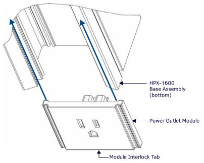
FIG. 27 Inserting the Power Module into the HPX-1600 Chassis
