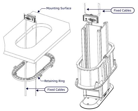
**FIG. 7** Fixed Cable Passing Through Ring, Table and Into the HPX-1600 Assembly Note the direction of the screw bosses, as indicated in FIG. 8:
