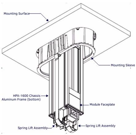
FIG. 18 Completed Assembly Latched in the Closed Position
