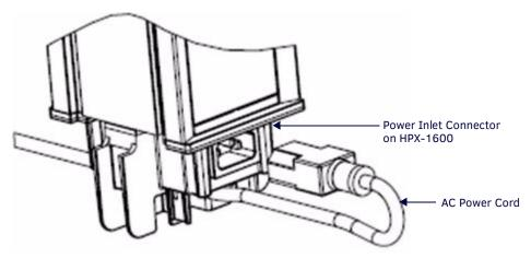
FIG. 25 HPX-1600 - Power Inlet Cord Removed
