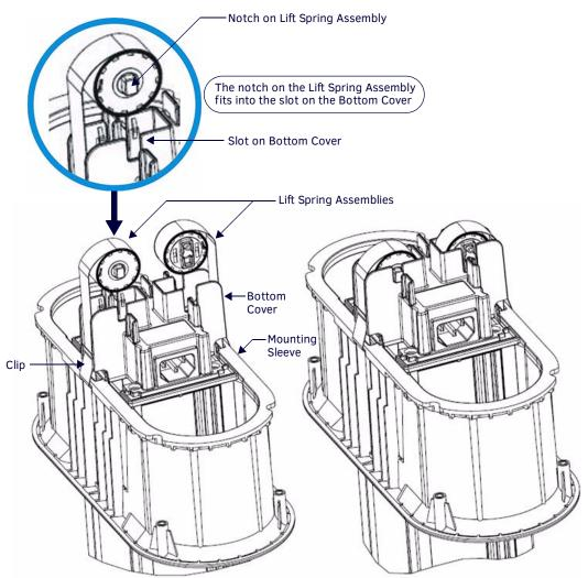
FIG. 17 Inserting the Lift Spring Assembly Into the Bottom Cover
