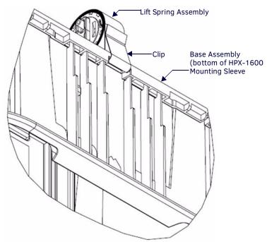
FIG. 16 Lift Spring Assembly Clipped to Main Sleeve
