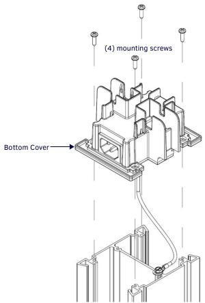
FIG. 9 Installing the Bottom Cover
