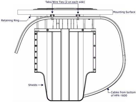
FIG. 23 Secured Service Loop
