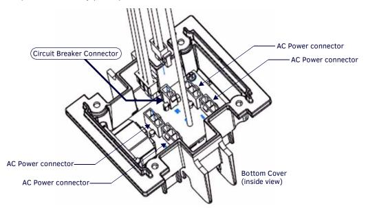
FIG. 13 Bottom Cover - Connect Each AC Power Module to the Power Inlet Assembly
