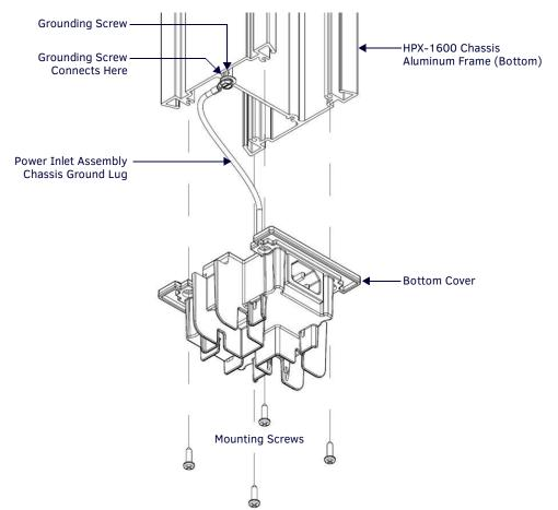
FIG. 14 Installing the Bottom Cover
