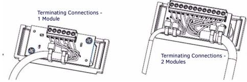
FIG. 6 Terminating Connections of 1 or 2 HPX Modules
