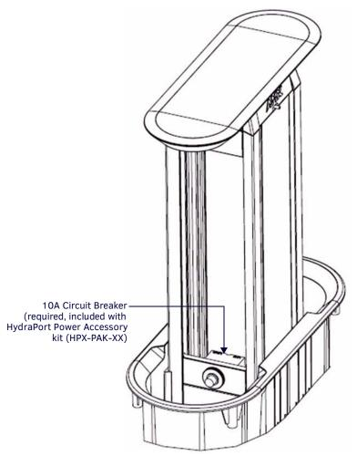
FIG. 28 10A Circuit Breaker Module Positioned Just Below Mounting Surface Level
