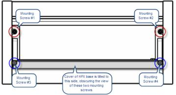
FIG. 2 HYDRAPORT BASE ASSEMBLY (SHOWN MOUNTED) - MOUNTING SCREWS LOCATIONS
