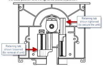
FIG. 3 HYDRAPORT BASE ASSEMBLY (SHOWN MOUNTED) - MOUNTING SCREWS LOCATIONS
