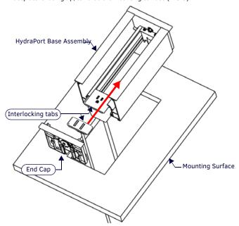
FIG. 5 INSTALLING THE HPX-N102-USB-PC MODULE
