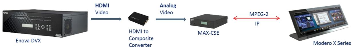
Fig. 3 Example of networked MPEG-2 video streaming to a Modero X Series touch panel
