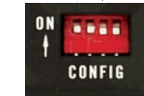
FIG. 1 CONFIGURATION DIP SWITCH
