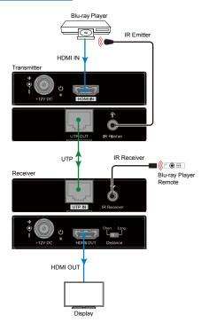
Note: Connect a broadband IR receiver to IR Receiver port and an IR emitter to IR Flasher port.
