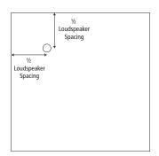
D. Remaining loudspeakers are arranged on a square grid pattern using the Loudspeaker Spacing distance.
