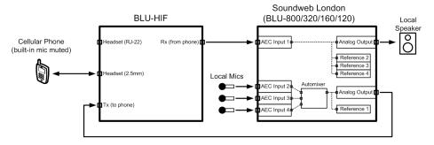
Figure 3: Wiring Diagram – BLU-HIF Headset Jacks
