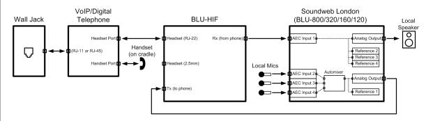
Figure 2: Using the BLU-HIF with a Phone Equipped with a 2.5mm TRS Jack
