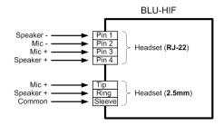
Caution: Do not connect to both jacks simultaneously. Doing so risks damaging the connected devices. Before connecting to either jack, ensure that the internal jumper is set to the appropriate position. By default, the BLU-HIF ships with the jumper in the Headset RJ-22 jack position. For more information on setting the internal jumper, please refer to the BLU-HIF Installation
