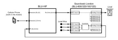
Figure 3: Wiring Diagram – BLU-HIF Telephone Headset Jacks
