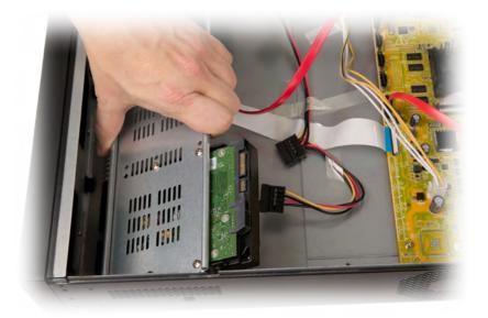
Remove the mounting bar by lifting the rear side, then pulling the entire bar away from the front of the recorder.
