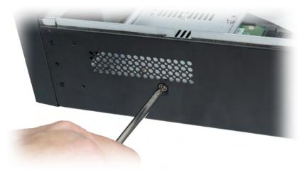
Remove the two black screws that hold the mounting bar in place. They are on the exterior of the unit, one at each side of the recorder.
