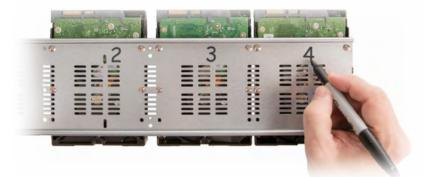
Line up the holes in the mounting bar over the drives, then use four of the screws supplied with the recorder to secure each drive in place.
