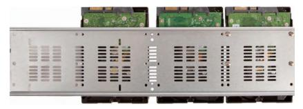
Lay the new hard drives to be installed side by side on a flat surface with the power and SATA ports facing the same direction and the circuit board on top.
