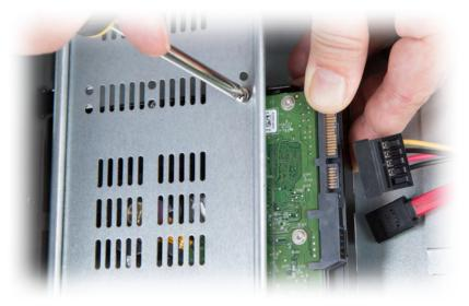
If you are only inserting one additional drive and are working with a larger recorder case, you might be able to install the new hard drive(s) without removing the mounting bar.
