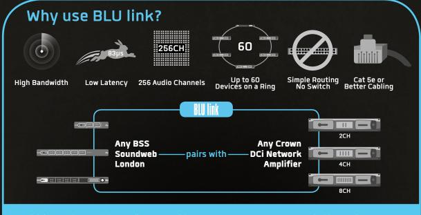
BLU link is not only a standalone audio transport, it's complementary! To save on costs and add convenience, run AVB CobraNet, or Dante through a BSS Soundweb London and convert audio to BLU link. BLU link enables an easy and flexible range of audio solutions through its increasing presence in HARMAN products.
