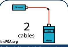
6. For double-ended testing, plug in two appropriate SC cables or two LC cables with adapters, one into OLS and one into OPM, with SC connectors or LC to SC adapters into OPM and OLS ports.<sup>1</sup>
