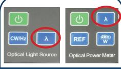
1. Select correct light source for fiber type being tested (SM = single mode or MM = multimode; labeled above screen on left). Turn on both light source (OLS) and power meter (OPM).
