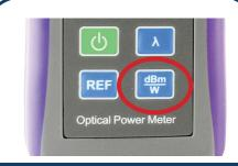
3. On the OPM, press the "dBM/W" button until dBM is the unit listed to the right of the main screen read-out (see step 1B image).
