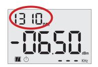
1A. Wavelength on the OLS is displayed in the upper left corner of the screen. Set to desired value (press wavelength key.)
