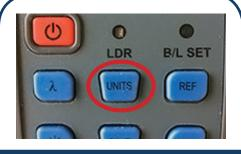
3. On the OPM, press the "UNITS" button until upper right portion of screen is blank and dBM is listed to the right of the main screen read-out (see step 1B image).
