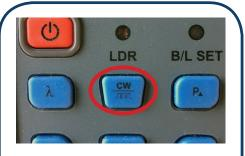
2. On the OLS press CW button until 0Hz displays in upper right of the screen (see step 1A image).
