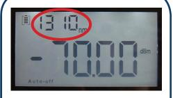
B. The OPM should be set to same wavelength as the OLS unit. Press the wavelength button until desired value appears.
