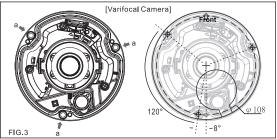
Adjust the pan, tilt, and azimuth of the camera to the desired location (FIG.4). Adjust the zoom and focus for the best image, and tighten the screws after the adjustment for manual varifocal models (Fig.4).
