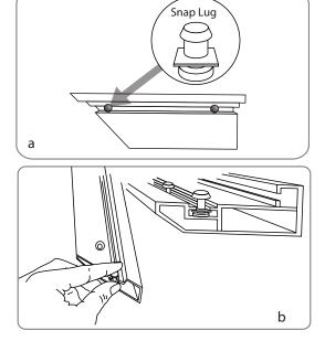
• The snap lugs line up with the arrow decals on the frame tubes. Alignment is not critical at this stage of the installation. Note that the screen is supplied with 2 extra snap lugs; should you lose or break a snap lug, one of the spares is a convenient replacement.
