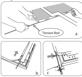
• Line up the snap lugs and the screen material with the frame and press the snap lug through the corresponding hole in the material. Some adjustment and re-adjustment is often necessary; this is normal. Note that the tensioning rod goes to the outside of the snap lug (See Diagram 4).
