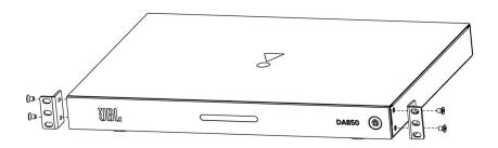
2. Install into rack and connect cabling.
