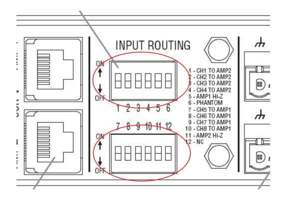
Step 3: Input #1 will now play on both AMP channel outputs and each output will maintain independent level control.
