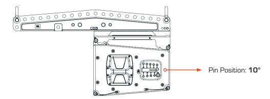
**REVERSE FRAME:** Reverse frame installation with the Extension Bar extending to the front of the array. Allows for additional up-tilt range and maximum load capacity.
