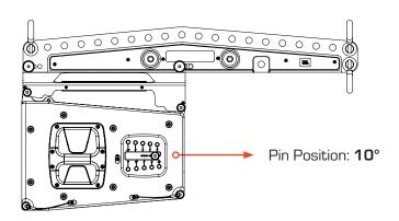
**REVERSE:** Extension Bar extends to the front of the array for additional up-tilt range. Supports limited number of cabinets.
