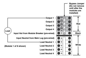
Torque Terminal Blocks from 3.5 - 5 in-lbs (0.4 - 0.57 Nm)
