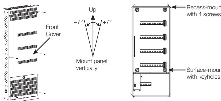
**3. Mount rough-in panel** using one of the following methods (mounting hardware is not provided):
