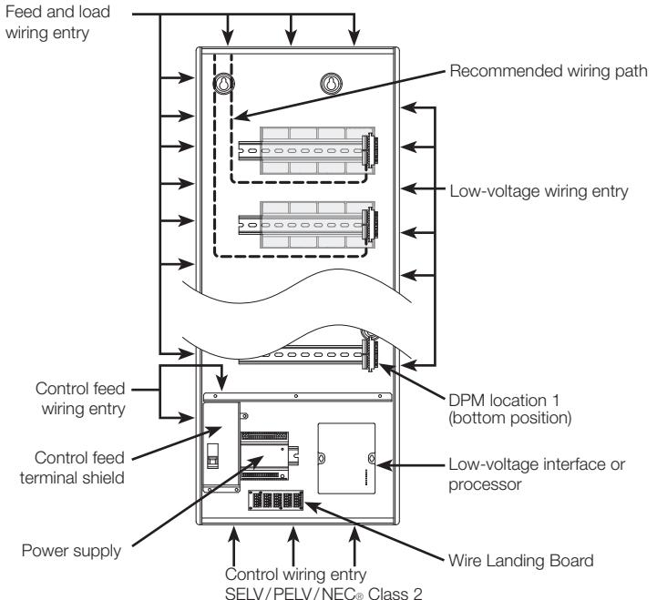
**5. Control feed wiring (control panels only).**
