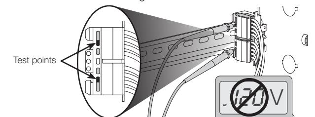
Install modules on the right side of each row. 5-position wire connectors and holders can be removed from the DIN rail row but should not be discarded so that they are available for future use. Each DPM controls up to 4 loads.
