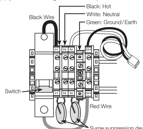
For increased system reliability, HomeWorks QS processors can be powered by an uninterruptible power supply (UPS) that incorporates overvoltage protection, brown-out protection, and battery backup. When selecting a UPS, allow 240 VA of capacity for each processor on the UPS. A single large UPS for all processors is better than an individual UPS for each processor. This prevents inconsistent system operation on battery backup if the individual UPS units power down at different times.
