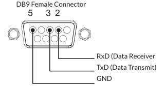
FIGURE 4: RS-232 (DB9) Pin Configurations
