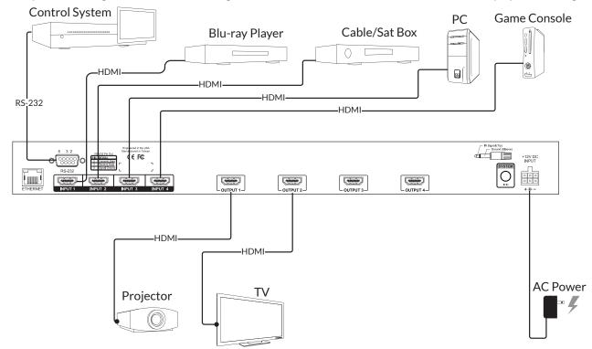
FIGURE 3: B-120-HDMATRIX-4x4 Installation
