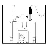
• Connect the 4 pin mini-XLR cable into the "MIC IN" of the body pack.
