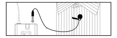
Important Note: Due to the distance between the talker's mouth and the microphone, lavaliere microphones are not designed for use in spaces where the talker is being reinforced in the same room - such as training rooms. Using them in these applications will often result in feedback due to the higher gain necessary for proper pickup. For these applications, the single ear hook and double ear hook microphones are recommended.
