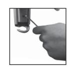
2 Mark both edges of the stud to help identify the exact center (see illustration).
