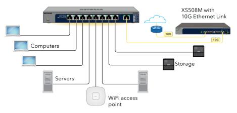
**NOTE:** We recommend that you use a Category 6a (Cat 6a) cable or higher-rated cable for 10-Gigabit Ethernet connections, and a Category 5e (Cat 5e) cable or higher-rated cable for other Gigabit Ethernet connections.
