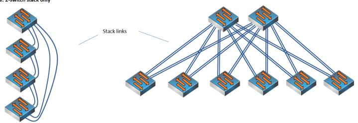
1G models: up to (4) 10G ports per switch can be used for stacking (depending on inter-switch links oversubscription requirements)
