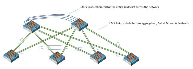
"Core" models: up to (16) 100G, 25G, or 10G ports per switch can be used for stacking (depending on total multicast requirement in the network)
