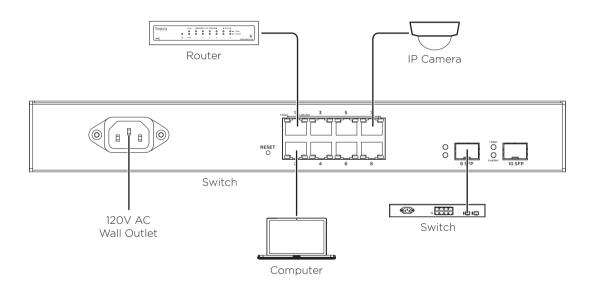
NOTE: Connect SFP ports using Araknis SFP adapters for RJ45 or multi-mode fiber cables. SFP adapters sold separately.
