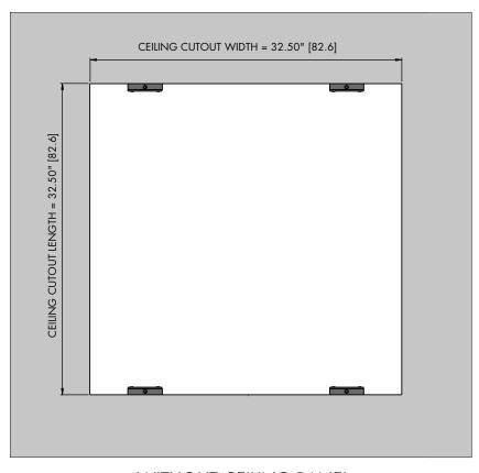
WITHOUT CEILING PANEL [USE FOR CEILING CUT-OUT DIMENSIONS]
