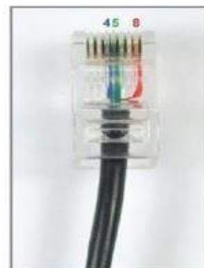
Close-up View of RJ-45 Pins
