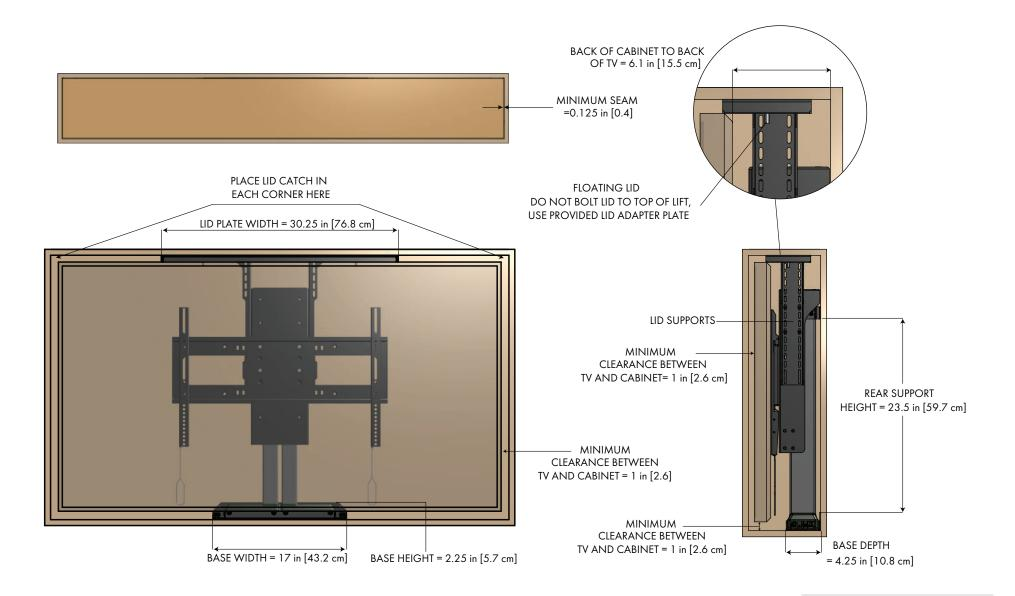
NOTES: 1. LID SUPPORTS ALLOW LID PLATE TO BE ADJUSTED FLUSH WITH UNDERSIDE OF LID 2. LID ADAPTER PLATE ALLOWS LID TO FLOAT WITH THE USE OF LID CATCHES 3. MINIMUM SEAM CAN BE REDUCED TO 0.0625 in [0.2 cm] WITH A 45 DEGREE BEVEL ON THE EDGES OF THE LID NEXUS<sup>21</sup>
