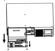
Remove the four battery panel screws, set the cover aside, and pull the battery tray from the front of the UPS.
