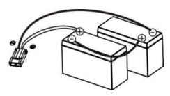
Replace the batteries in the tray. Wire the new batteries as shown above.
