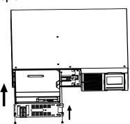
After swapping the batteries, replace the battery tray in the UPS and reattach the battery cover. Tighten the screws securely.
