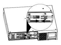
Connect the battery wires.
