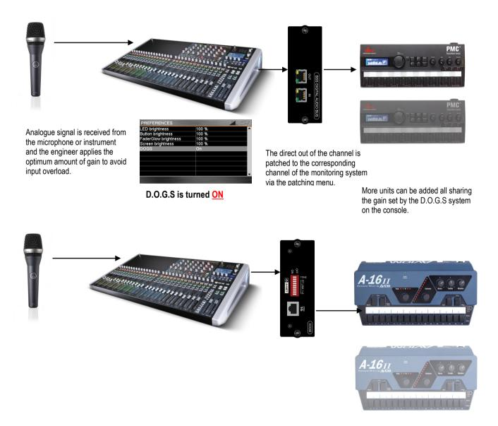
The systems portrayed above are proven methods of enabling musicians to alter their own instrument settings or monitor mix levels without being affected by the gain on the master console.
