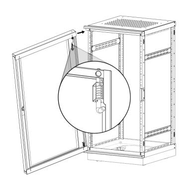
Note: The door may be installed for left- or right-hand swing. The hinge brackets are held on by 1 screw in each corner. The brackets are also slotted so that they can be adjusted for optimal door fit.
