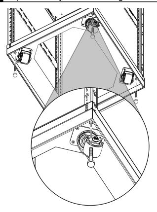
Note: Lowering the leveling feet restricts the steering rotation of the casters. If the feet are being used, position the rack before installing equipment.
