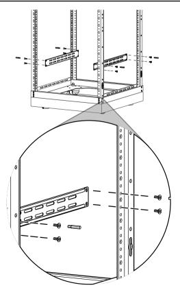
Note: The side bars are not required for structural support and can be mounted at any height. (Two of four included bars are pictured.) 4 Optional: Adjust the leveling feet.
