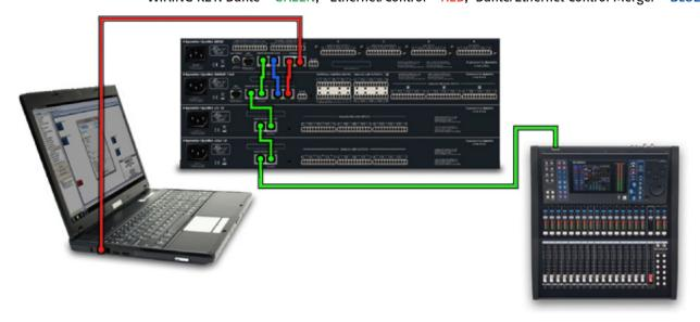
Once the Dante and Ethernet control networks have been merged, the DVS and SymNet Composer or SymVue can both function simultaneously from the same laptop.
