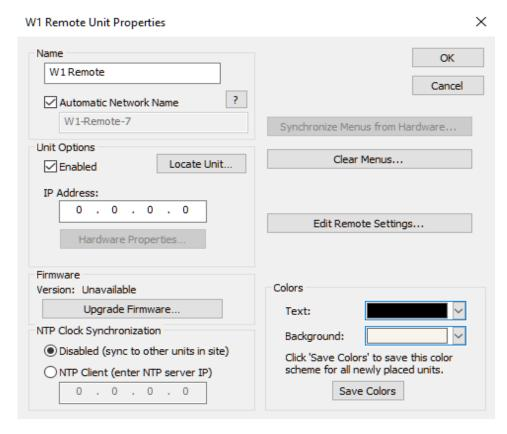
Network configuration of W Series remotes is done in the same manner as Symetrix DSP network settings are configured, using the unit properties dialog box.
