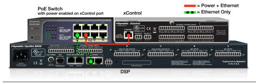
Connection to PoE switch/network without PoE injector.
