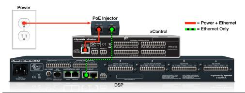
Direct connection to DSP using PoE injector.
